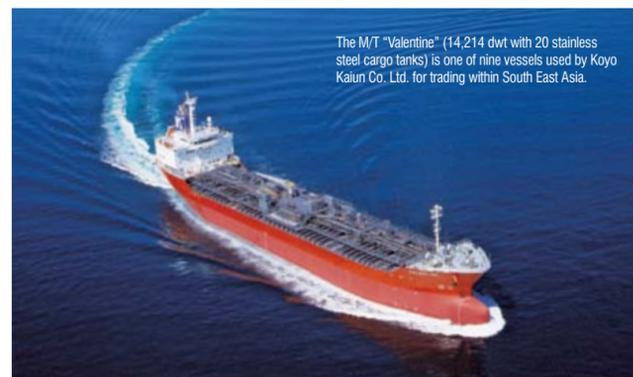
The M/T "Valentine" (14,214 dwt with 20 stainless steel cargo tanks) is one of nine vessels used by Koyo Kaiun Co. Ltd. for trading within South East Asia.
